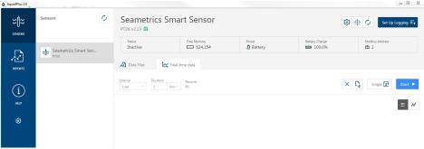
To start real-time readings click Start, readings default to table view. To switch to Real-time graphing view click the graph icon  $\checkmark$
